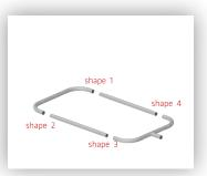
4. Connect the aluminum frame together by matching the simlilar shapes on the stickers.
