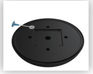
2. Tightly screw in the plastic washer to prevent leaking.
